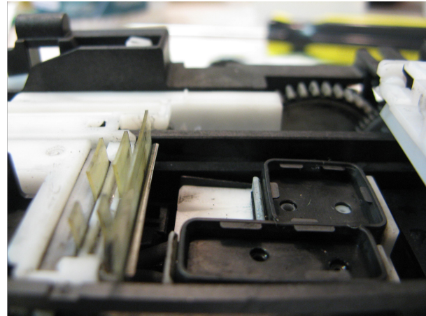
Figure 9 – Suction holes exposed suction units are down
