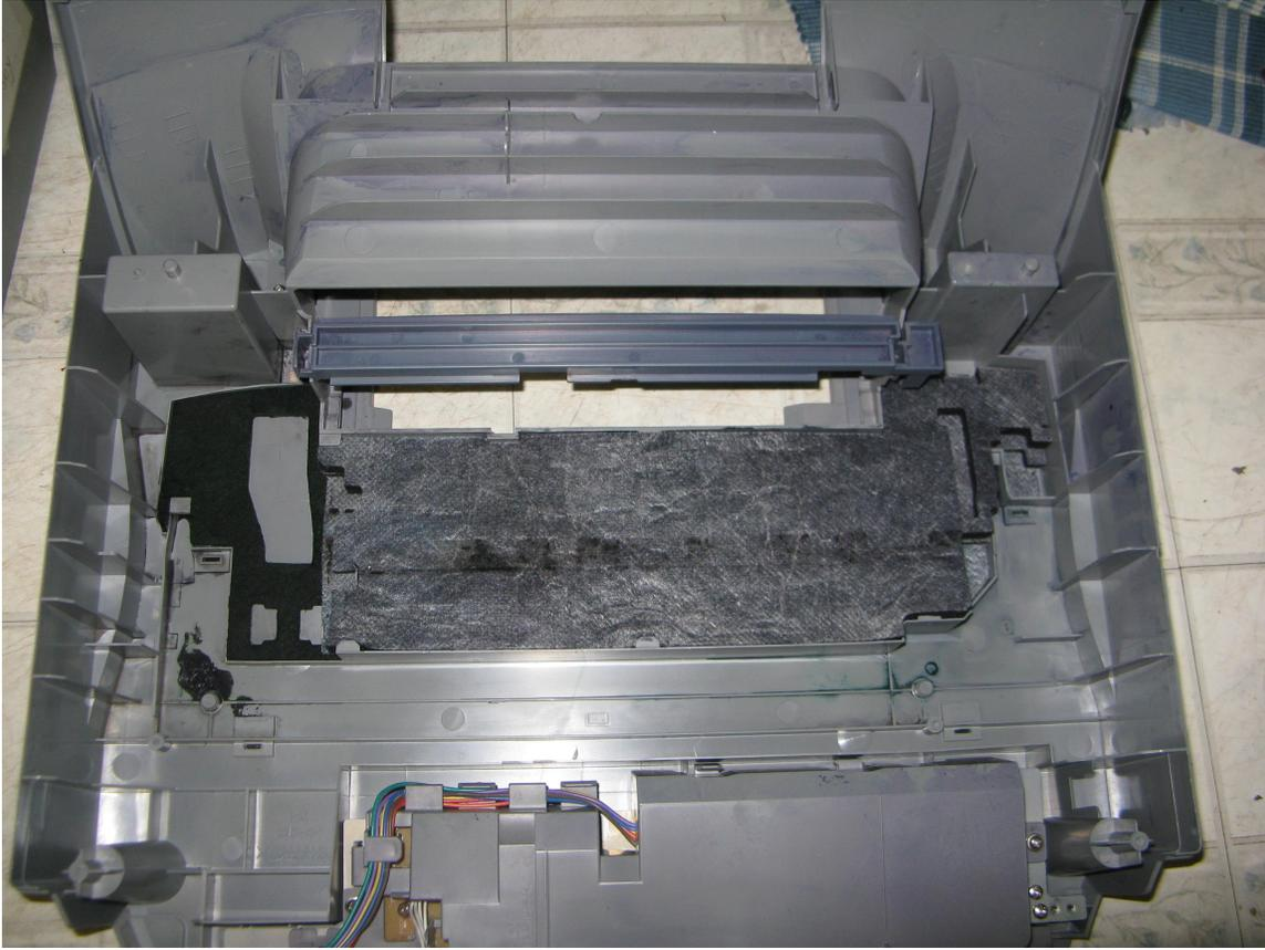
Figure 24 – Cleaned up ink blotters back in bottom of case
