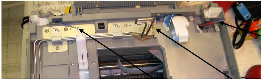
Figure 13 – Three ground screws
