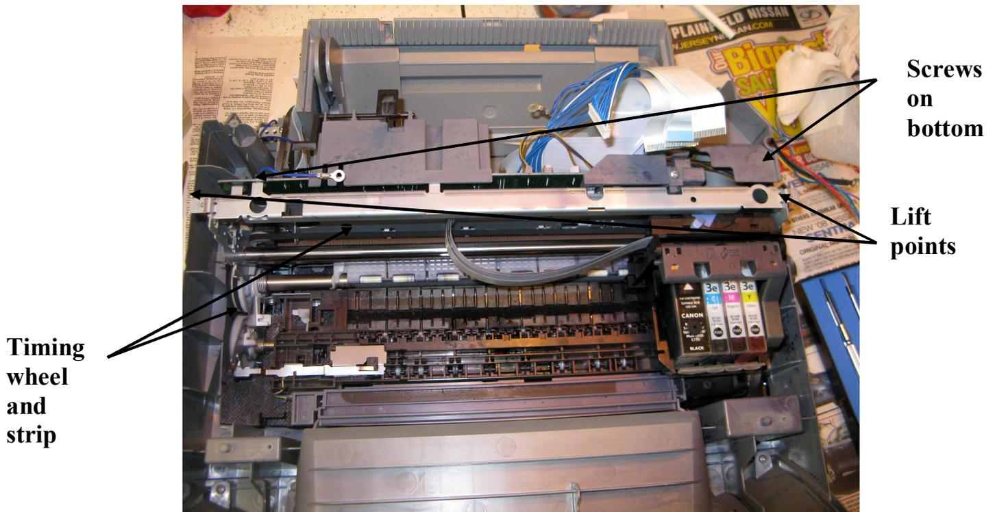
**Figure 15 – Print and paper feed assembly**
