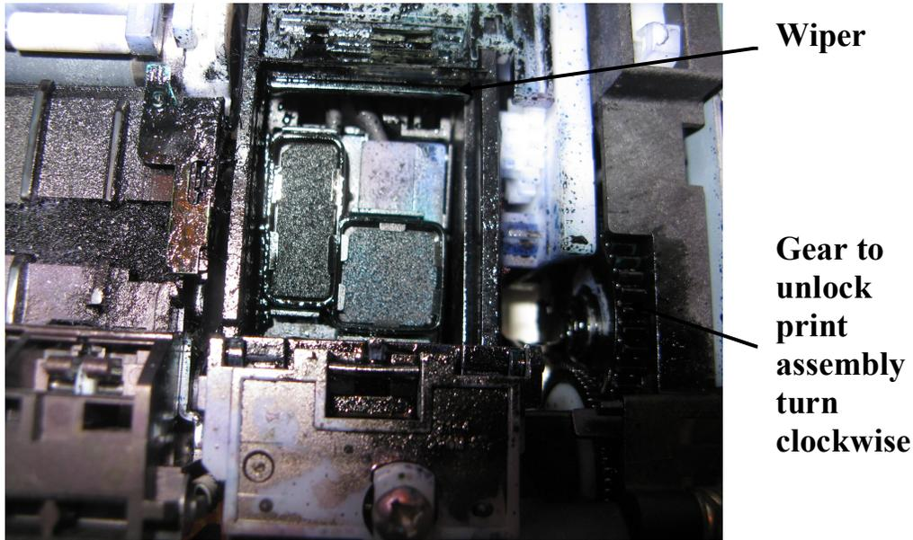
**Figure 20 – Top of purge unit showing ceramic pads. Suction holes beneath. Wiper at top.**
