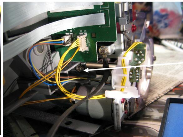
**Figure 23 – Screws for taking off the page feeder**
