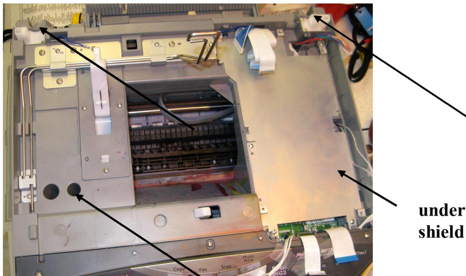
Figure 14 – Screws to take out middle frame unit
