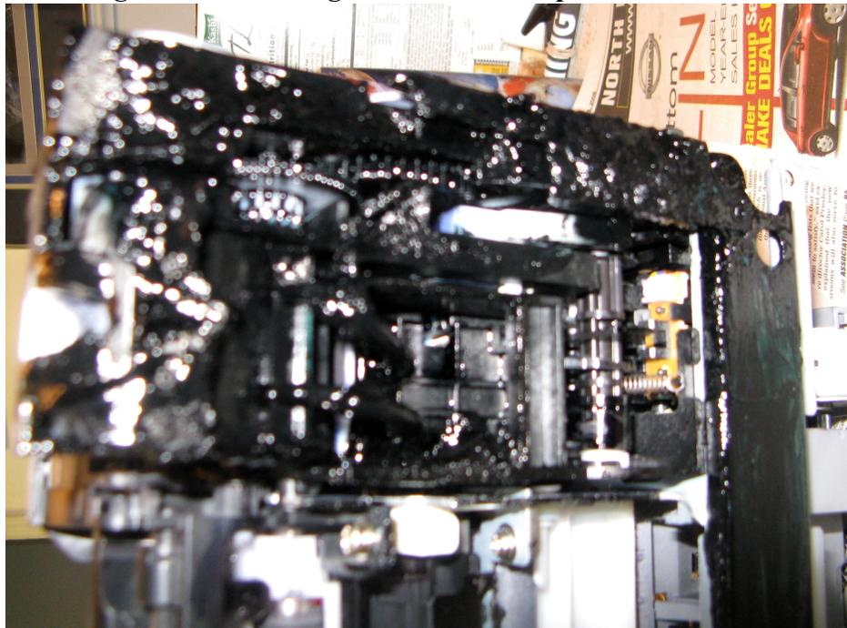
**Figure 17 – Bottom of purge unit covered in ink**
