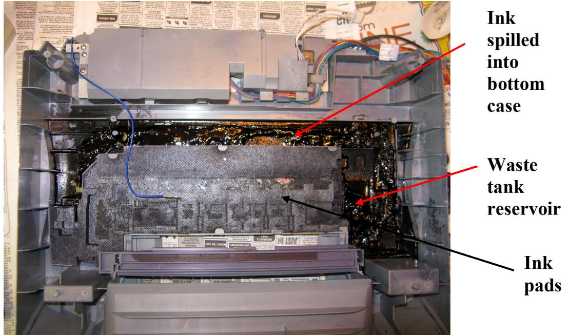
**Figure 16 – Showing ink in bottom of printer**
