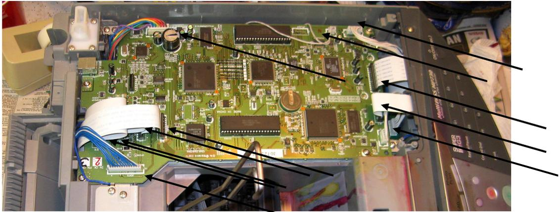
Figure 9 – SPCNT board connectors
