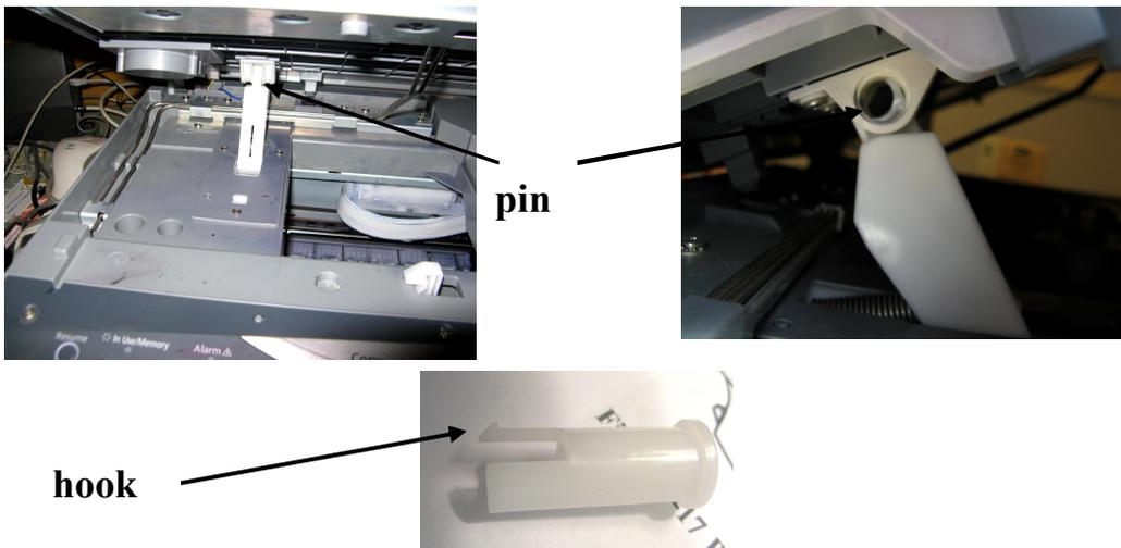
**Figure 8 – Joint and pin location**
