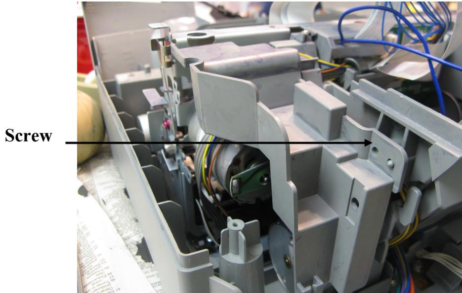
**Figure 22 – Take off cover to get a purge unit wires**
